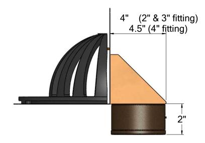
16 oz copper flashing soldered to spout, attached to 2", 3", or 4" bronze no-hub fitting
