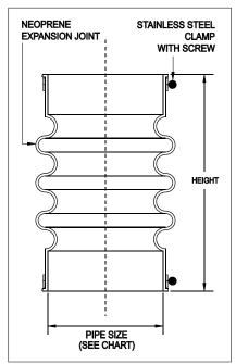
For each model, the compression is 1", expansion is 1/2" and rotation is 10 degrees.
