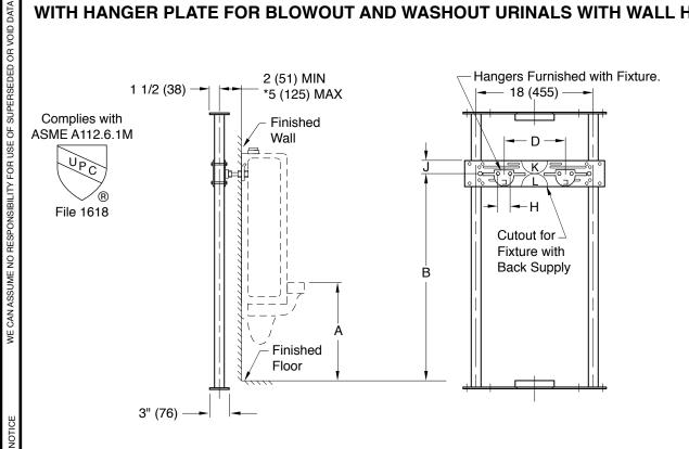
NOTE: \*This dimension can be increased when fixture support is to be installed behind the wall (specify when required and wall thickness).
