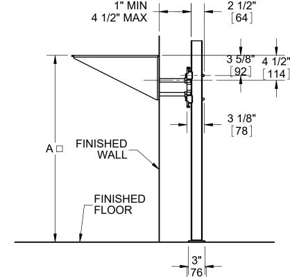
RECOMMEND ALL FEET BE SECURED TO FLOOR WITH 1/2" BOLTS AND ANCHORS BY OTHERS.
