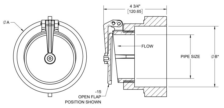
\* MEETS ASTM A-74 XH CAST IRON SOIL PIPE STANDARD
