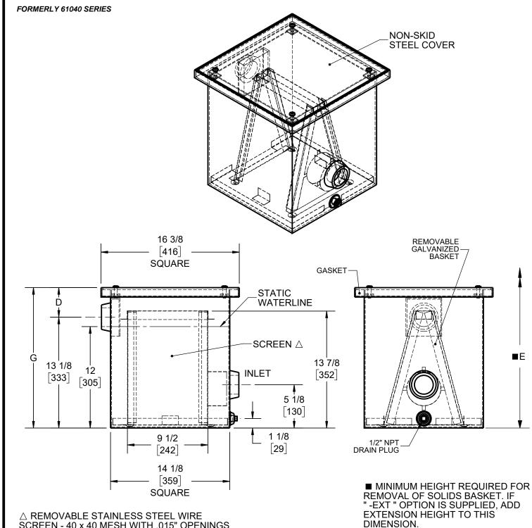
△ REMOVABLE STAINLESS STEEL WIRE SCREEN - 40 x 40 MESH WITH .015" OPENINGS
