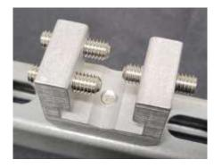
3. Set the upper rail assembly on the seams at the desired location with the RoofClamps centered over the seams, check that the rail is level and straight. Tighten the RoofClamp top bolts with a micro torque wrench to 90 inch pounds. Push down on the Unistrut while tightening all RoofClamp set screws to 90 inch pounds.
