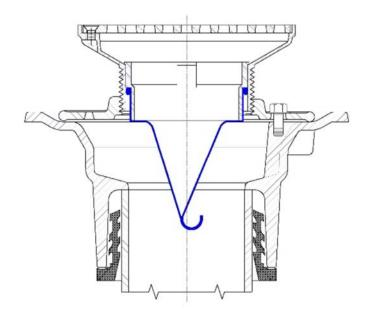
**Regularly Furnished:** Elastomeric trap seal device with fitting for internal tailpiece or pipe installation.
