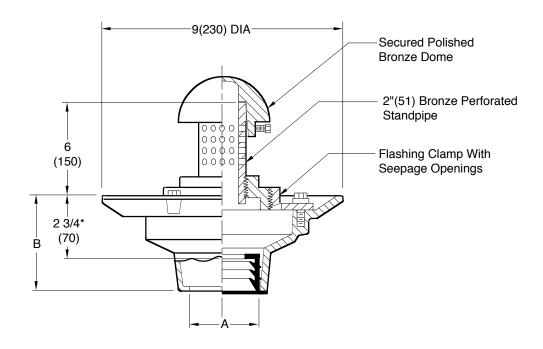
Fig. 2680C . . . CAULK OUTLET Fig. 2680Y . . . NO-HUB OUTLET
