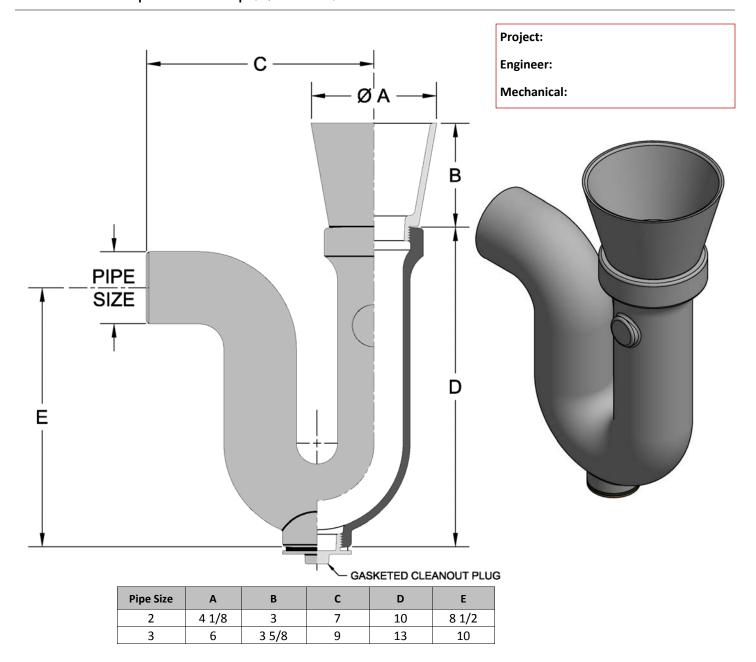
Regularly Furnished: Cast iron deep seal trap with bottom bronze, gasketed plug, & 1/2 IPS pipe connection with plug.
