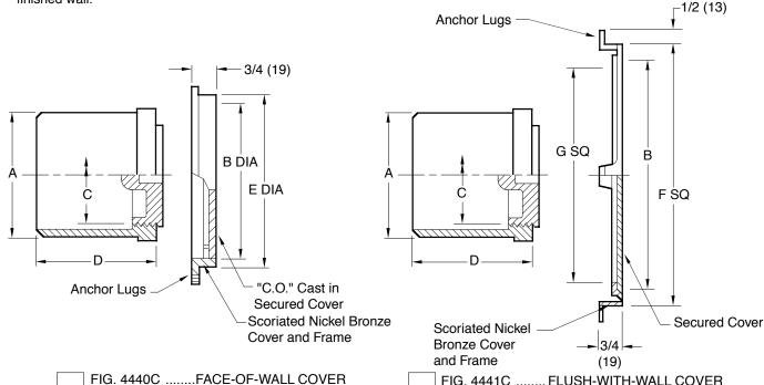
FIG. 4440C ......FACE-OF-WALL COVER
