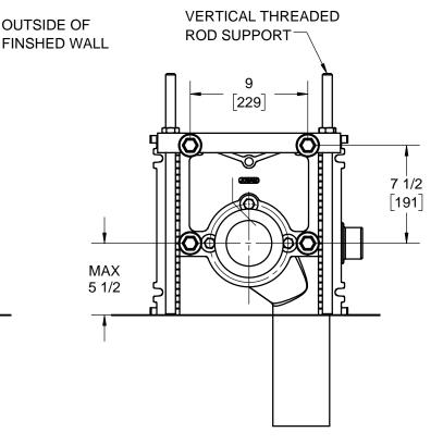
RECOMMEND CONCRETE ANCHORS WITH 750 LBS. PULL-OUT FORCE EACH
