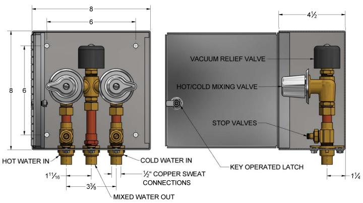
**Regularly Furnished:** Surface mounted stainless steel remote water supply box with hot & cold water shut off valves, screwdriver stops, vacuum relief valve, hinged cover with cylinder lock, & 1/2 copper sweat connections.
