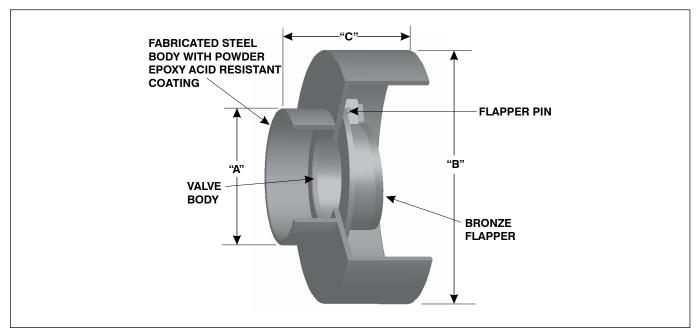
Note: The BV1280 terminal valve is used at the end of sewer lines to prevent backflow into areas that require draining.
