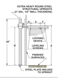
Note: Wall supported fixture mounting plates must be securely affixed (with suitable hardware by others) to a wall fully capable of bearing the weight of the plate and fixture.
