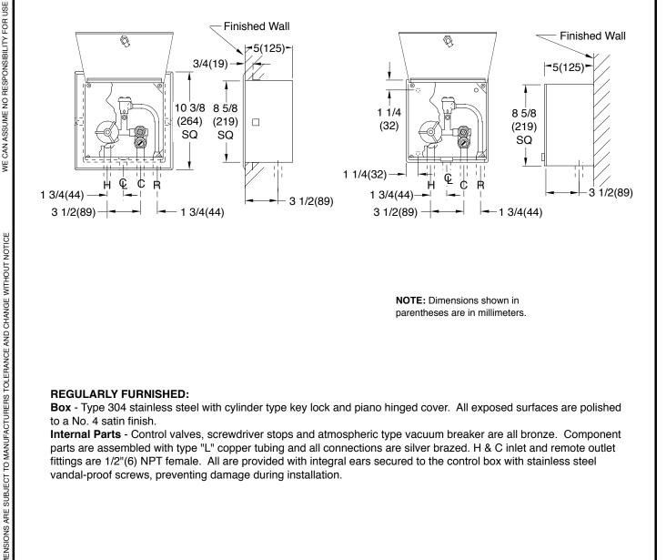
NOTE: Dimensions shown in parentheses are in millimeters.
